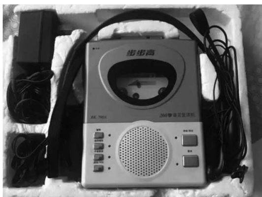
FIG. A typical configuration for a repeater: the upper blue part to play cassettes, and the lower grey part for the digital interface. (Shasha, 2019)
